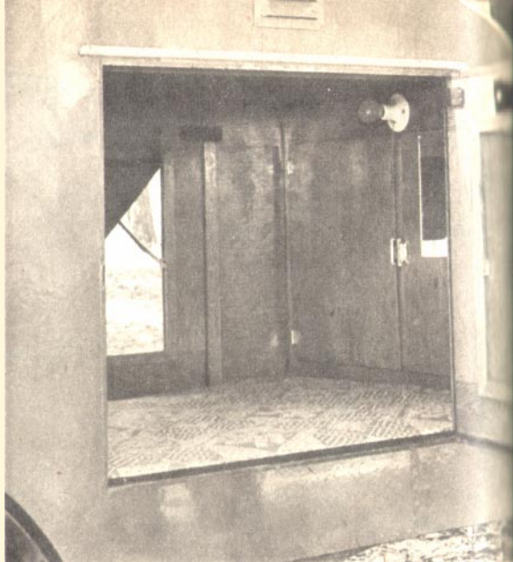
Forward end view of interior. Storage compartment doors must be high enough to clear bedding.
