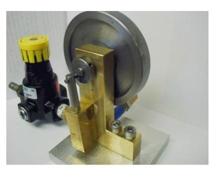
Here's a small oscillating steamer built from plans found on the internet. The original source site has shut down (and we have not gotten a response from the site webmaster) so we've redrawn the plans with a few minor changes (and aluminum could be used as a substitute for the brass). The engine uses an "L" shaped frame and "upside down" layout (the crank is over the piston). We added a
