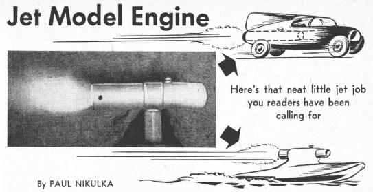
THIS ram-jet motor is presented here by special request of the hundreds of SCIENCE AND MECHANICS' readers who saw the photograph of it which appeared in the Readers' Round Table (p. 26, Oct. '48, S & M). It can be made from a few odd pieces of aluminum which you may obtain from a sheet metal shop or the nearest hobby center. Also the tools required are within the scope of most experimenters. All set? Let's go!
