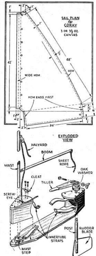
with two 1/4 in, bolts. Notch the rudder post as shown to take the blade. Make up the tiller from on KULLER a piece of 1/4 in. oak fastened to the rudder post with one ¼ in, bolt and wingnut,
