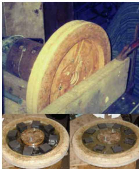
Rotor mould being made and used
