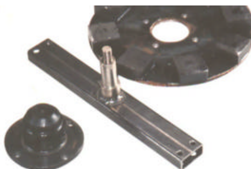
Spine, shaft, hub and magnet rotor
